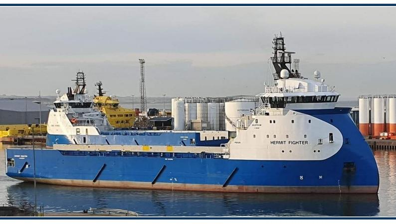
The vessel was built and designed by ULSTEIN as a platform supply vessel. The hull form, with the ULSTEIN X-BOW®, combined with diesel electric propulsion system, ensures the best performances with regard to fuel consumption, sea keeping, station keeping, and speed. The main propulsion system comprises two azimuth pulling thrusters, each driven by frequency controlled variable speed electric motor. The Vessel is manned for 24/7 continuous operation.
